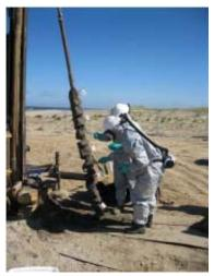
Before the start of the experiments each pilot test cell is characterised in detail regarding geology and initial contamination distribution.
