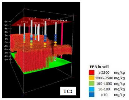
Figure 7: Distribution of EP3 concentrations above 2000 mg/kg in the test cell 2 (TC2).
