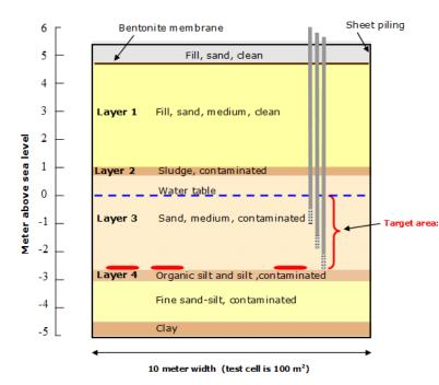
The characterisation shows that the geology at the site is relatively uniform to the investigated depth of elevation -2,8 m. The geology is characterised by the following layers:
