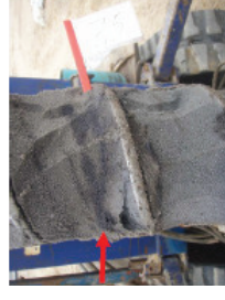
Figure 8: Free phase on top of a narrow fine-grained horizon in TC2-4
